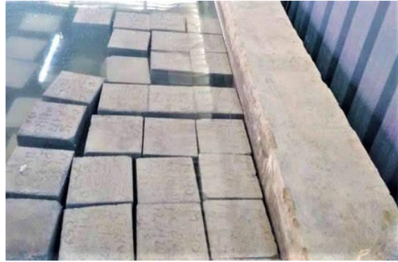
Figure 4: Curing of Concrete Samples
