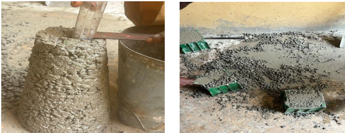
Figure 1: Slump Test using Inverted Cone
